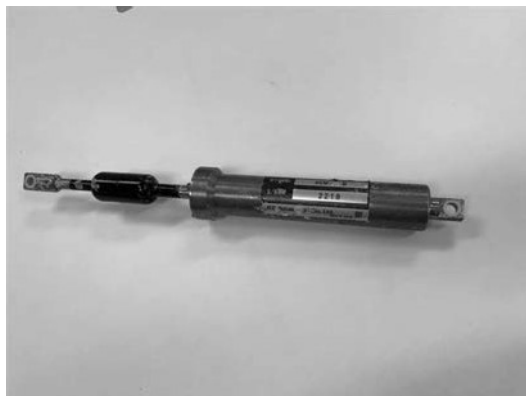
Figure 1. Tidal current measurement device (AEM-USB, JFE Advantech Co., Ltd.)
