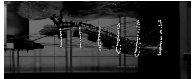
Figure 2 The trajectory of the membrane with 0.6 m/s current flow
